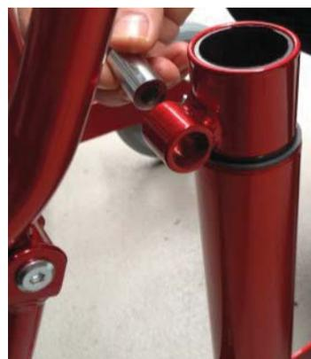
The new threaded rod is somewhat longer than the red holder to give free access to the special fitting
