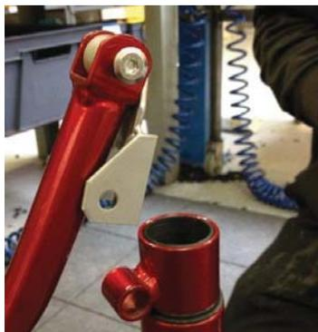
The new threaded rod, the bushing and the allen screw head shall be used to mount the special fitting on the lower frame and the wide open part of the new fitting
