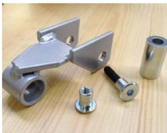
Loosen the tilt bar from lower frame. The existing threaded rod, the bushing and the allen screw head shall be used to mount the special fitting on the tilt bar.
