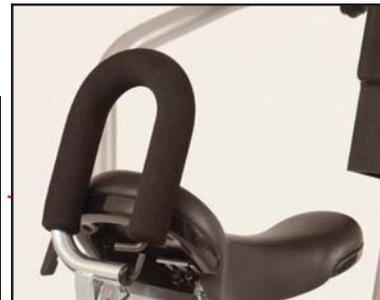
The rear stop behind the seat can be adjusted in depth. First lift up the rear stop and tilt it backwards. This reveals an Allen screw inside the U-profile. When the Allen screw is loosened, the rear stop can be slid forwards or backwards in the external tube. After adjustment, re-tighten the Allen screw.
